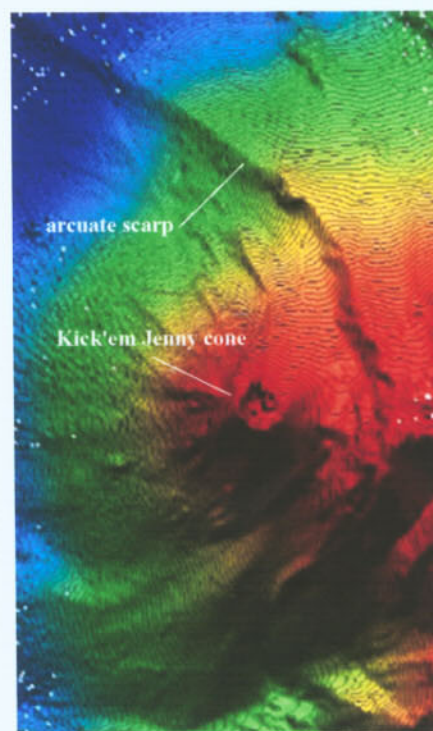
Fig.2. Morphology of Kick'em Jenny volcano as revealed by a multi-beam survey by NOAA's R/V Ronald Brown in March 2002. The survey shows that the modern cone of the volcano is nested within a larger horse-shoe shaped depression, probably formed by slope failure and debris avalanche generation. Crater diameter is approximately 300 m and the contour interval is 10 meters. Depth to the crater rim is about 190 meters.
