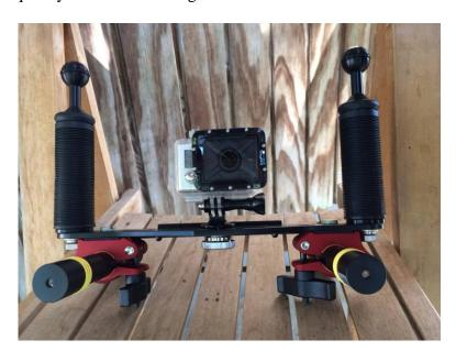
**Figure 4.14.3.**Materials used for rigging the video camera and underwater lasers for calibration of images
