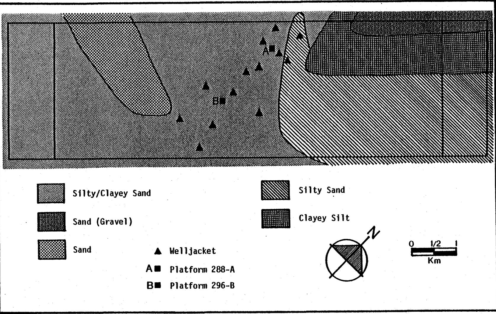
Fig. 5. Sediment distribution in the Buccaneer Gas and Oil Field (Anderson and Schwarzer 1979).
