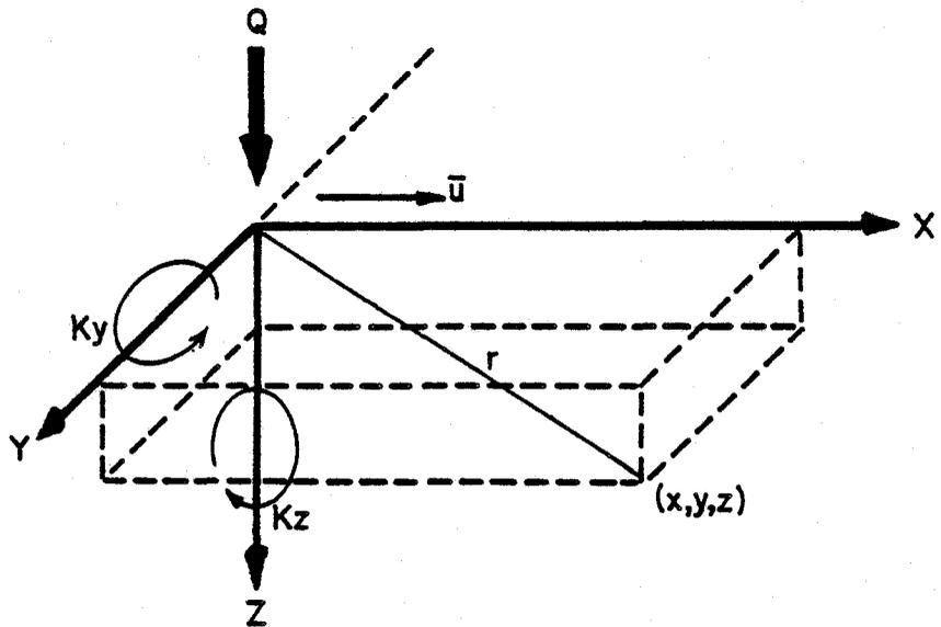
Schematic of idealized dispersion from continuous point source of effluent. The ambient current is flowing in the x direction with velocity  $\bar{u}$  (m/sec).  $K_y$  and  $K_z$  are eddy diffusion coefficients ( $\text{m}^2/\text{sec}$ ) in the horizontal and vertical directions respectively.  $Q$  is the rate of effluent introduction at the source ( $\text{m}^3/\text{sec}$ ).  $r$  is the distance (m) from the source to the point  $(x, y, z)$ .
