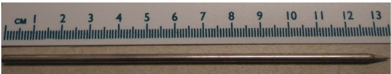
Figure 7. -- Photo of the stainless steel hollow loop tag applicator/piercing needle (Hallprint) used in Method 2. Entire applicator is approximately 13 cm in length.
