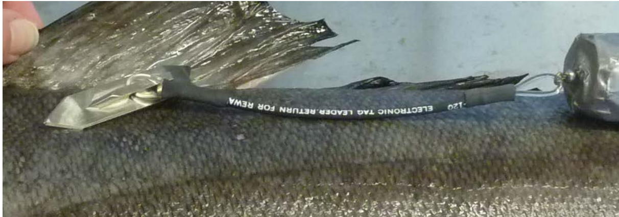
Figure 3. -- Photo of a completed Method 1 tag tether displayed dorsally on a sablefish for comparison. This tag tether should be approximately 3 to 4 inches in length.
