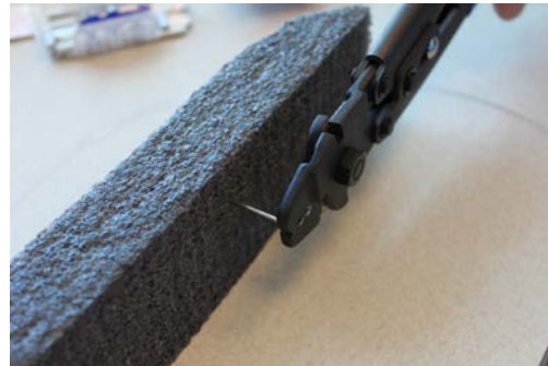
Figure 1. Insert piercing needle through dorsal musculature using the smallest hole on crimping pliers.
