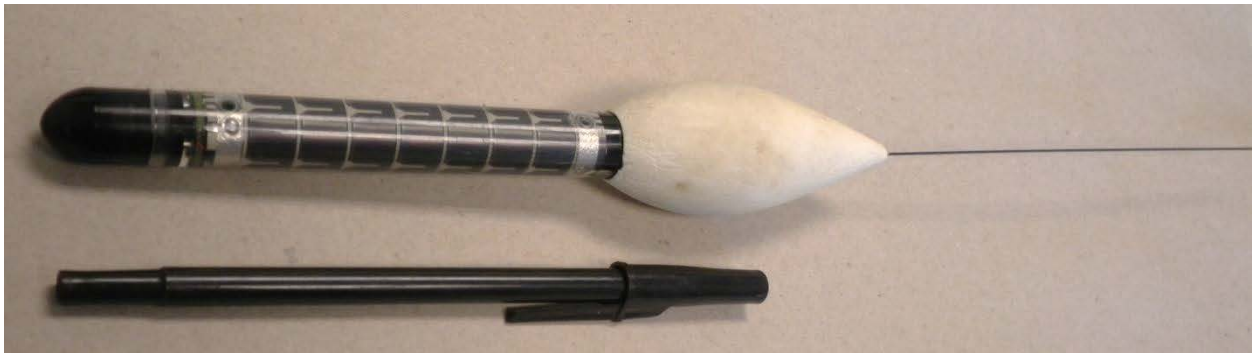
Figure 2. -- The Desert Star SeaTag-GEO next to a pen for size comparison.
