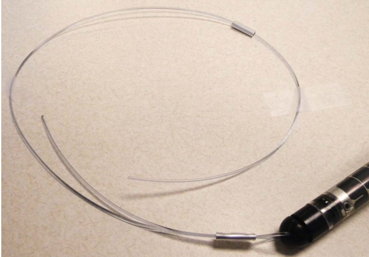
Figure 5. -- Method 2 tag tether before attachment to fish.
