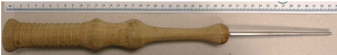
Figure 6. -- Photo of the tag applicator used in Method 1, consisting of a wooden handle with a stainless steel dart inserter (Hallprint) screwed in at one end. Entire applicator is approximately 43 cm in length.
