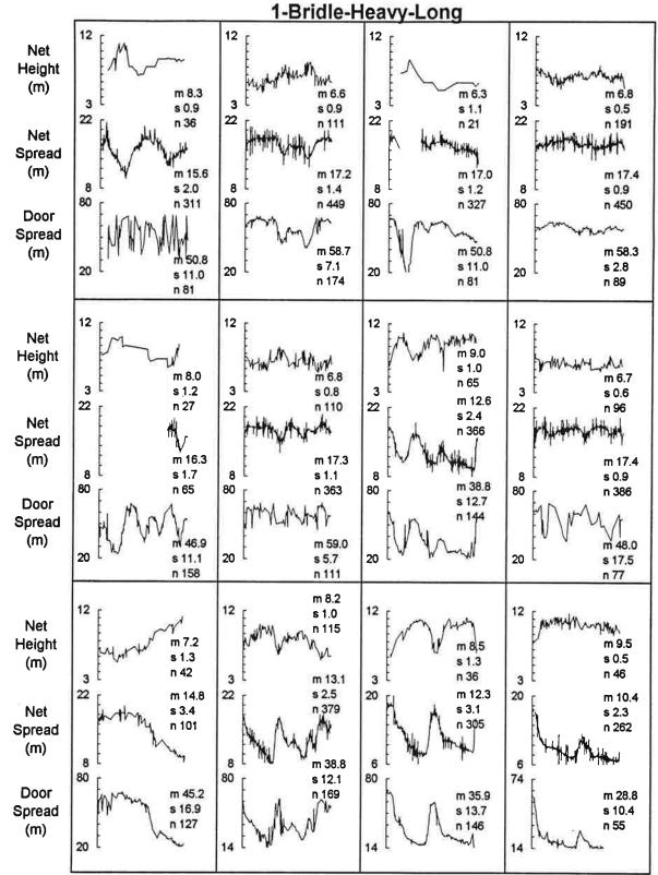
Figure 2.--Graphs showing SCANMAR net height, net width, and door spread during the course of each tow for the 1-bridle-heavy-long gear treatment (m=average, s=standard deviation, n=number of observations).
