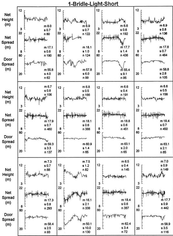
Figure 5.--Graphs showing SCANMAR net height, net width, and door spread during the course of each tow for the 1-bridle-light-short gear treatment (m=average, s=standard deviation, n=number of observations).
