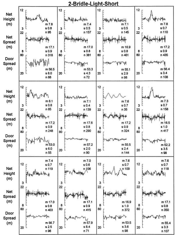
Figure 9.--Graphs showing SCANMAR net height, net width, and door spread during the course of each tow for the 2-bridle-light-short gear treatment (m=average, s=standard deviation, n=number of observations).
