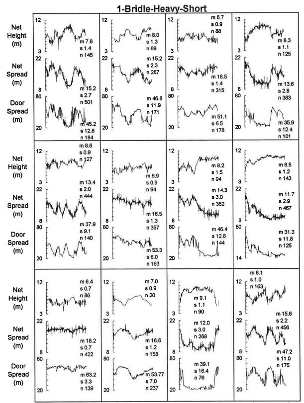
Figure 3.--Graphs showing SCANMAR net height, net width, and door spread during the course of each tow for the 1-bridle-heavy-short gear treatment (m=average, s=standard deviation, n=number of observations).
