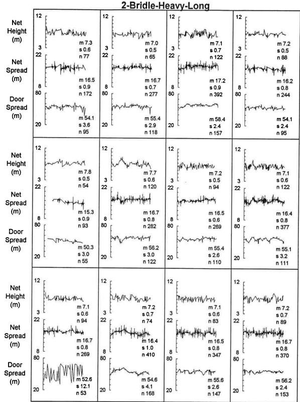
Figure 6.--Graphs showing SCANMAR net height, net width, and door spread during the course of each tow for the 2-bridle-heavy-long gear treatment (m=average, s=standard deviation, n=number of observations).
