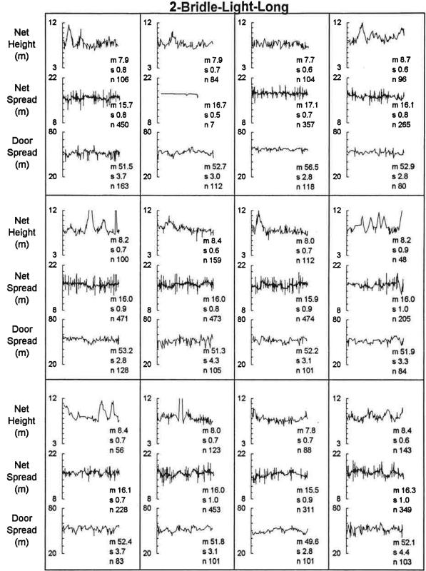
Figure 8.--Graphs showing SCANMAR net height, net width, and door spread during the course of each tow for the 2-bridle-light-long gear treatment (m=average, s=standard deviation, n=number of observations).
