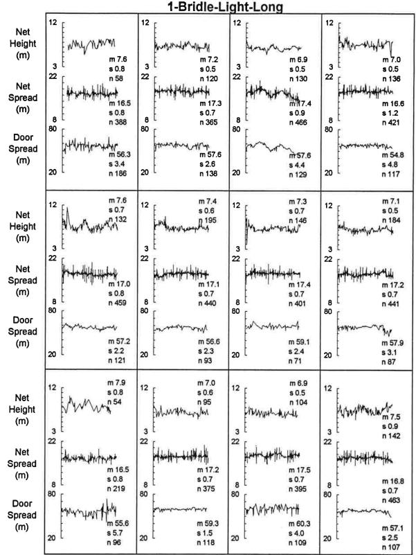
Figure 4.--Graphs showing SCANMAR net height, net width, and door spread during the course of each tow for the 1-bridle-light-long gear treatment (m=average, s=standard deviation, n=number of observations).
