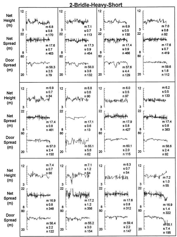
Figure 7.--Graphs showing SCANMAR net height, net width, and door spread during the course of each tow for the 2-bridle-heavy-short gear treatment (m=average, s=standard deviation, n=number of observations).
