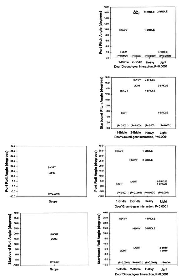
Figure 13.--Results of analysis of variance to test the effects of the gear treatments and their interactions on door attitude. Statistically significant effects (P<0.05) are with uppercase letters.
