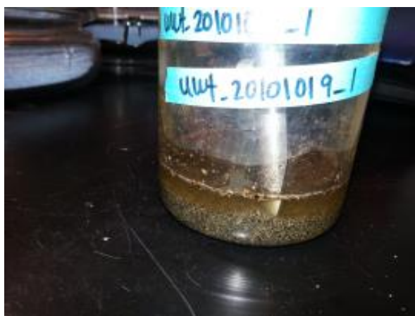
Figure 16. Lithium metatungstate is added to a sediment sample.
