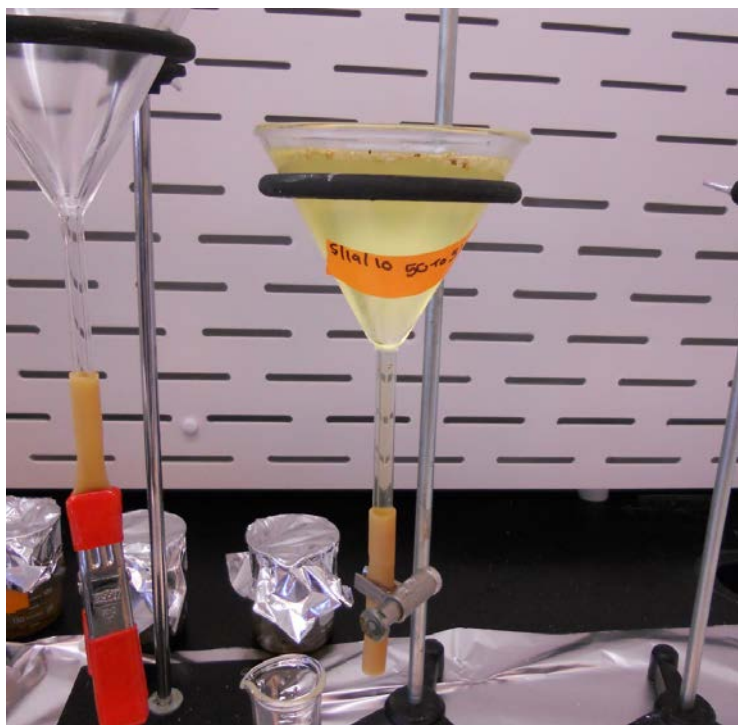
Figure 9. A sample is depicted in a glass funnel to separate plastic.
