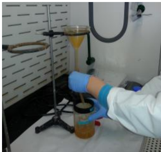
Figure 10. Floating material is drained into a custom sieve.
