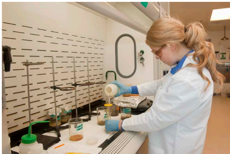
Figure 7. Addition of iron sulfate solution catalyzes the reaction.
